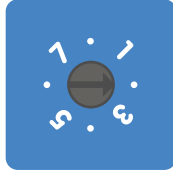
Rotary switch set to position 2
